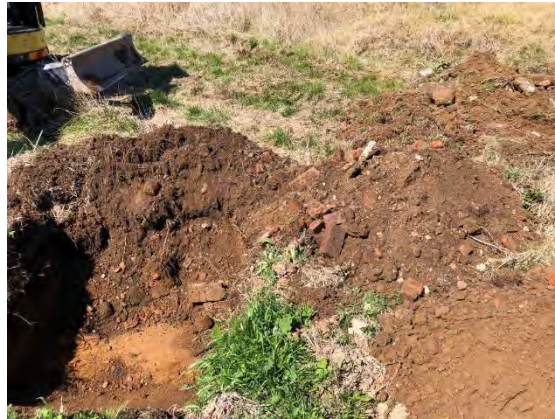
TP07 – soil intermixed with building demolition waste
