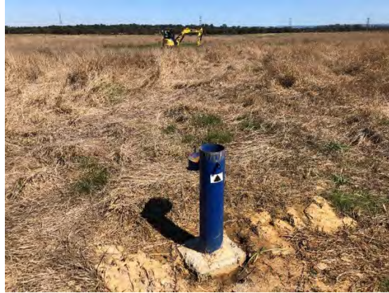
Existing groundwater monitoring well – located in the vicinity of TP05
