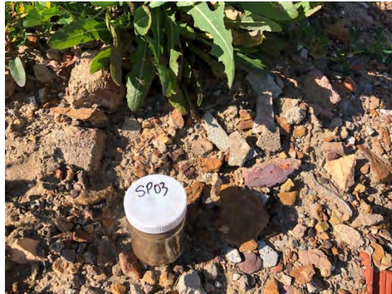
SP03 – asbestos materials identified on stockpile surface
